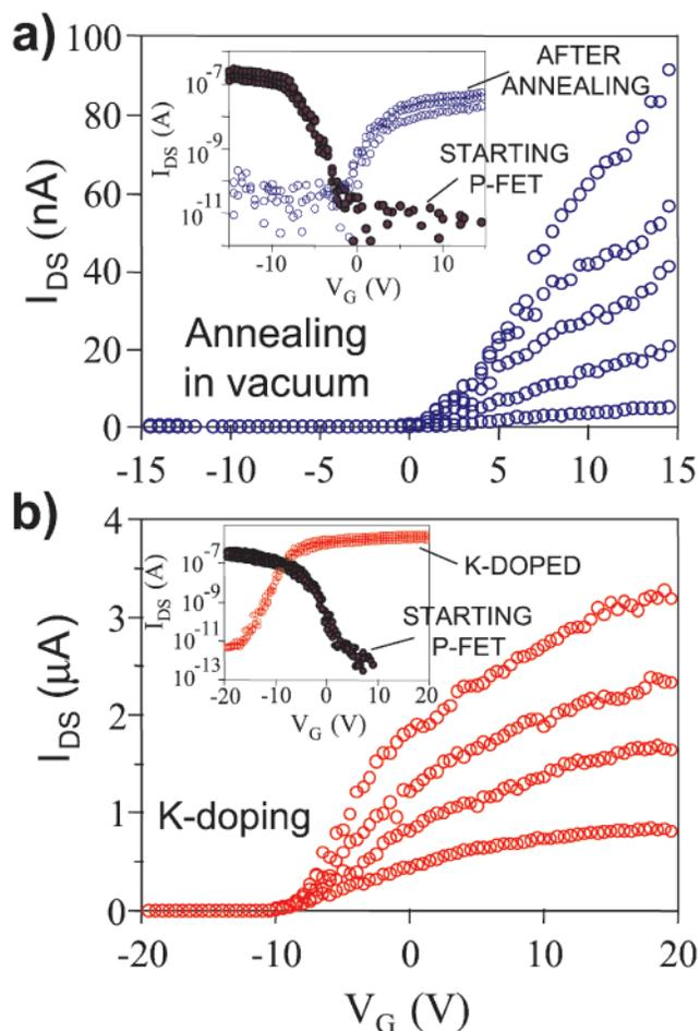
**Figure 1.** Electrical characteristics of n-type nanotube FETs made by (a) annealing the device in a vacuum at 700 K for 10 min and (b) doping with potassium. The curves are obtained at different values of  $V_{DS}$  starting at (a) 300 mV, step size 200 mV and (b) 200 mV, step size 200 mV.
