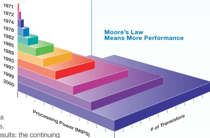
Processing power, measured in Millions of Instructions per Second (MIPS) has risen because of increased transistor counts.
