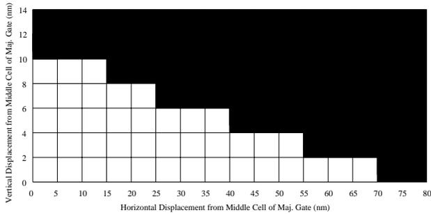
Fig. 3. A schmo plot showing pass (white) vs. fail (black) for the horizontal and vertical displacements of the horizontal input to a majority gate, such as Input B in Fig. 1(c).
