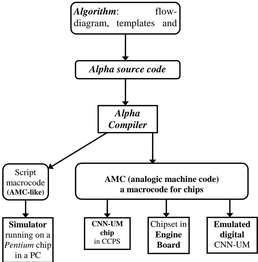
Figure 3. The levels of the software and the core engines
