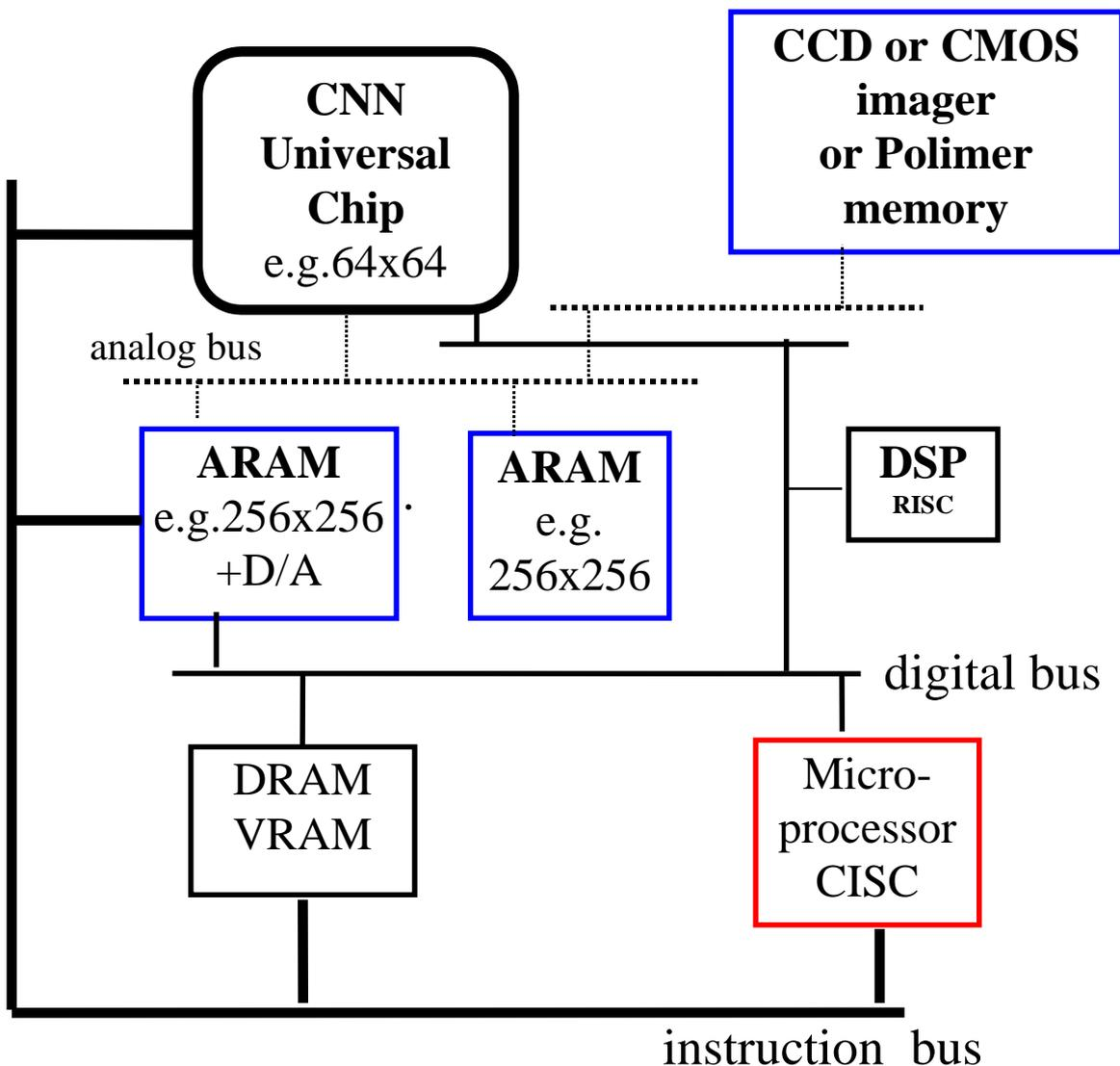
Figure 2. The CNN Chipset Architecture
